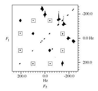
Fig. 4. 2D three-pulse *Q*-COSY Fz spectrum of 1 displayed at very low contour level (positive level). The intensity is multiplied by a factor of 8 compared with previous 2D contour plot. For such a level, we can see  ${}^2H-{}^2H$  correlation peaks (showed by the squares) and some residual on-diagonal peaks.
