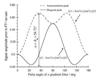
Fig. 2. Evolution of signal amplitude of autocorrelation and diagonal peaks as a function of the pulse angles of *z*-gradient filter for the 2D *Q*-COSY Fz sequence. At  $\alpha = \theta_{\rm m}$ , the autocorrelation signal is maximum while the diagonal signal is eliminated.
